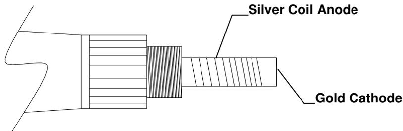
6. To clean the silver coil anode, soak the probe into 3% ammonium hydroxide solution overnight. After soaking, rinse with de-ionized water.
