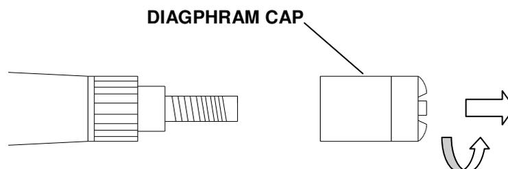
2. Half fill with new electrolyte into the (new) DIAGPHRAM CAP. Lightly tap the container to remove bubbles inside.
